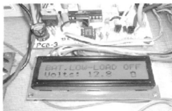
Lead-OFF, Battery-Low Condition
